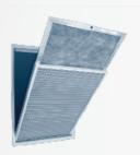
2. Clean any dust or debris from both sides of the filter using a vacuum cleaner, a soft dry cloth, or a soft brush. Do this on a flat surface to stop the frame from bending out of shape.
